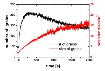
**Figure 5.** Number and size of crystallites as a function of time. 250 s after the quench from  $\Gamma=20$  to 80, the number of nuclei decreases again. This marks the time period, where the grains start to merge.
