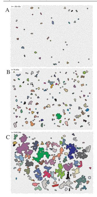
**Figure 4.** The Voronoi cells for particles recognized to be crystal-like are shaded. Colloids belonging to the same grain have the same shade. (A) In the fluid phase  $\Gamma=20$  some small clusters do appear but vanish within a few seconds. (B) Crystal grains of the 2D sample 77 s after the quench from  $\Gamma=20$  to 80. (C) Same area 1545 s after the quench—the grains touch each other (only grains which are completely in the field of view are plotted).
