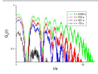
Figure 1. Log-log plot of the orientational correlation function for different time steps before and after the quench from  $\Gamma=20$  to 80. Before the quench the correlation decays within a few lattice sites, while after the quench it increases with time. We never observed an algebraic decay (linear curve in the log-log plot) which would be the signature of the hexatic phase.
